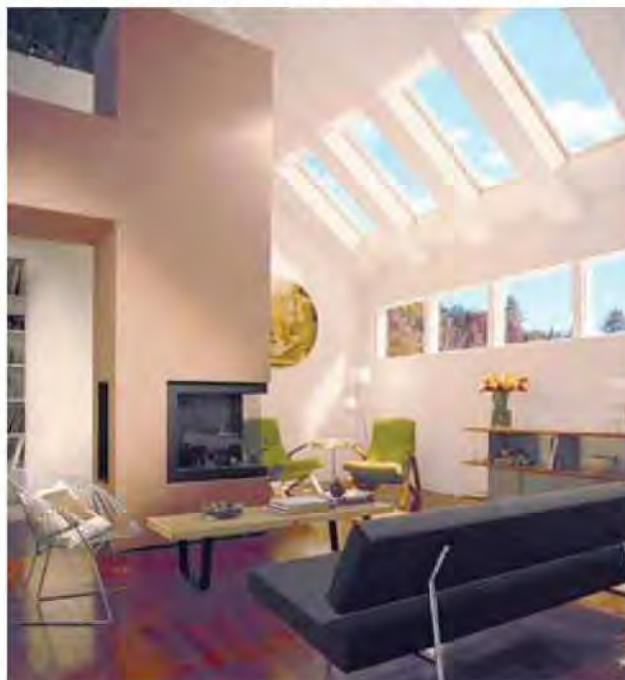
Skylights offer excellent daylighting and have the potential to displace much electric lighting, thus saving on lighting and, potentially, cooling energy.
